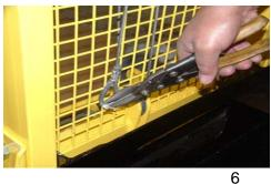
**Step 7.** Cut plastic tie holding lifting cable.
