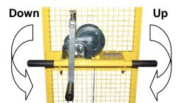
Turn winch crank clockwise to elevate the load, while watching for overhead obstructions. Turn winch handle counter clockwise to lower the load.
